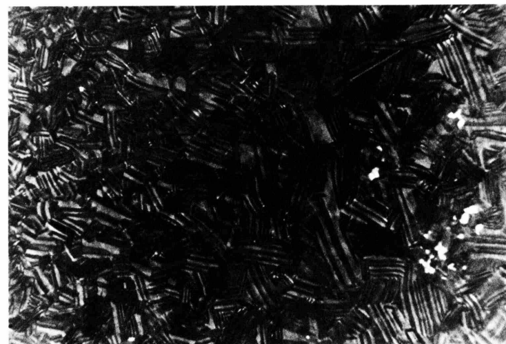
Fig. 3. BP I texture in an electric field. (Experimental conditions: cf. Figure 1.) Temperature 30.83 ^{\circ}\text{C} .
